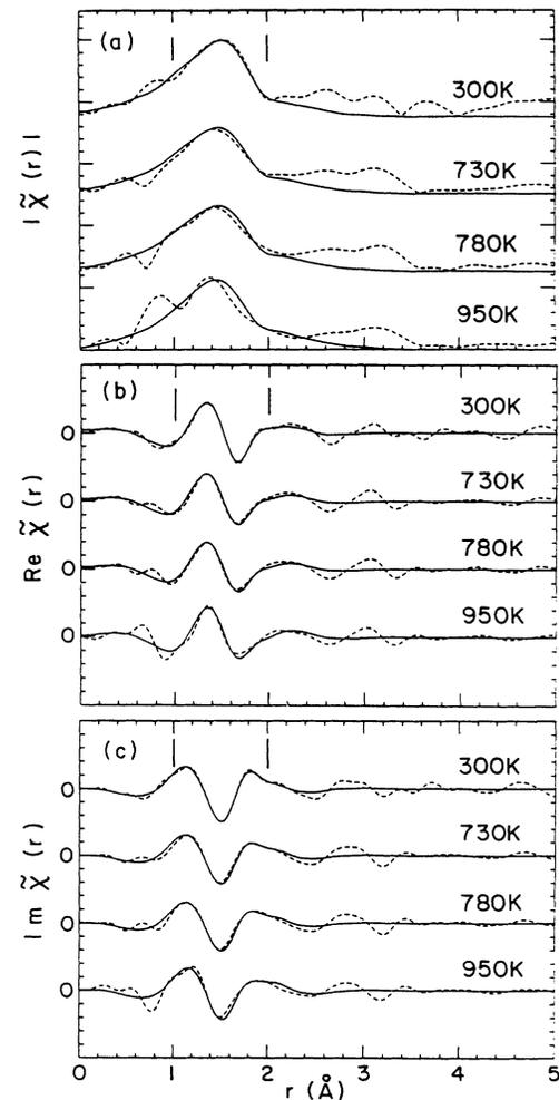
FIG. 6. The Fourier transforms of the Ti-edge XAFS spectra  $\tilde{\chi}(r)$  as a function of the distance to the probe  $r$ , for several representative temperatures. Dashed and solid lines represent the experimental results and the theoretical fits, respectively. (a) Absolute value, (b) real part, and (c) imaginary part. The temperatures are indicated in the figure. The vertical lines indicate the fitting range.
