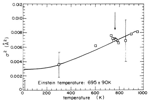
FIG. 7. The temperature dependence of the  $\sigma^2$  of the Ti to oxygen bond. They were obtained when this parameter was allowed to vary. The solid line is an Einstein fit to the experimental points. The transition temperature is indicated by the arrow.
