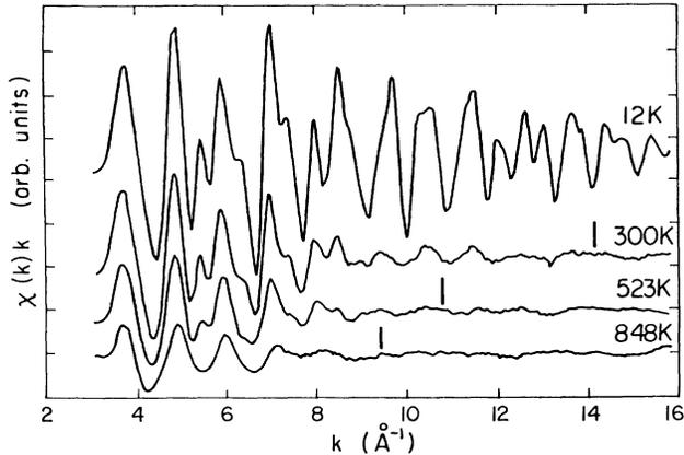
FIG. 2. The normalized Pb-edge XAFS multiplied by the photoelectron wave number  $k$  as a function of  $k$  for several representative temperatures. The vertical marks indicate the limits of useful XAFS data (see text).
