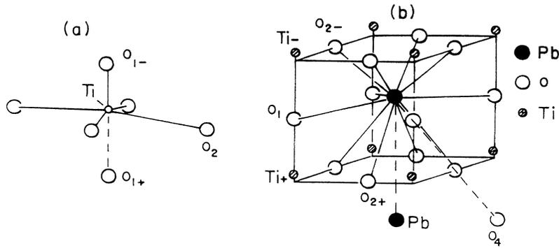
FIG. 1. Schematic structure of PbTiO<sub>3</sub> around each one of the probe atoms. (a) Ti, (b) Pb.
