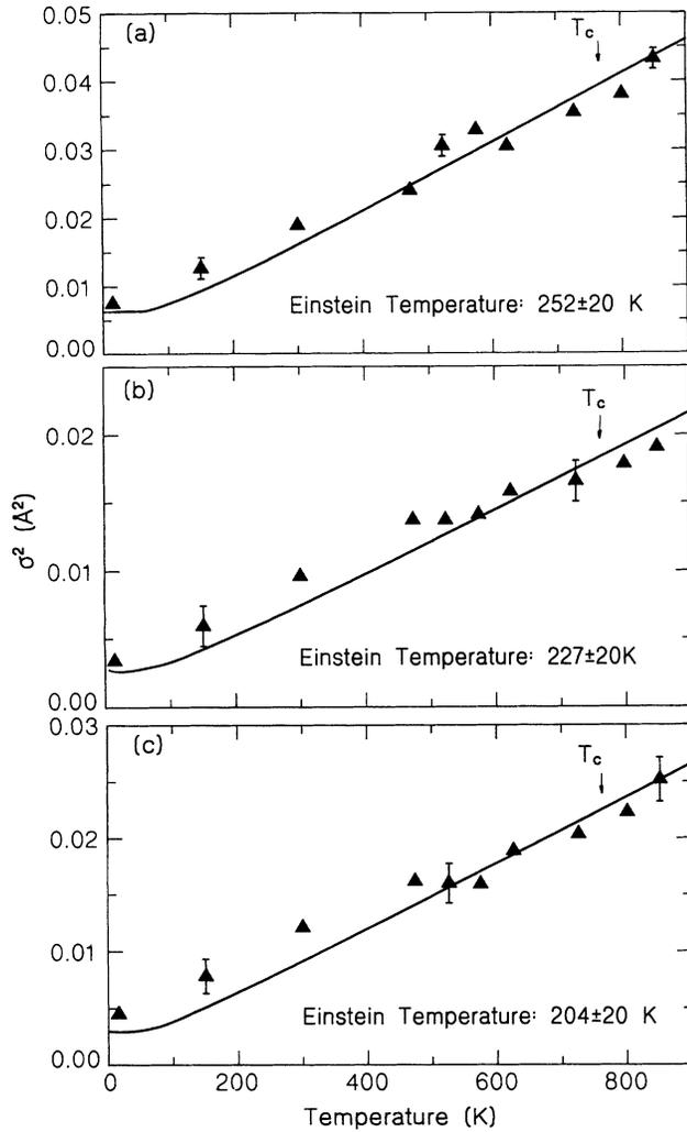
FIG. 8. The temperature dependence of Pb edge  $\sigma^2$ 's. The solid  $\Delta$ 's represent the experimental results. The solid lines are Einstein model fits to the data. The Einstein temperatures obtained are shown in the figures. (a)  $\sigma^2$ 's of the Pb to near oxygen bond. (b)  $\sigma^2$ 's of the Pb to near Ti bond. (c)  $\sigma^2$ 's of the Pb to far Ti bond.
