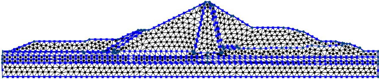
Fig. 2. Finite element mesh generated for the dam
