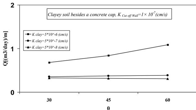
Fig. 8. Effect of  $\theta$  angle on the flow in connection No. 5
