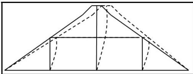
Figure 2b: 1<sup>st</sup> Mode (Shear)
