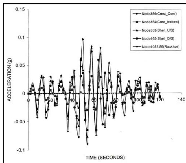
Figure 8: Acceleration at different nodes of the dam
