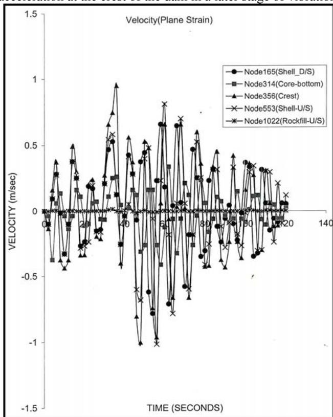
Figure 14: Velocity at different points in the dam
