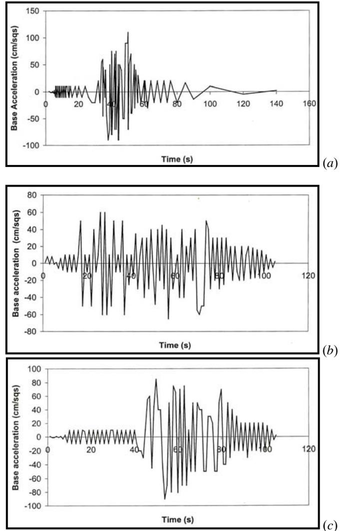
Figure 5: (a) N-S component (b) Vertical Component, and (c) E-W component of base acceleration data from Bhuj earthquake, Ahmadabad (26<sup>th</sup> Jan, 2001)
