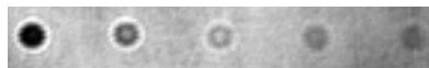
Fig. 10. One hundred-gigahertz images of 25-mm-diameter milled voids with different heights located in triple-slab SOFI panel at substrate obtained using the 6-mm-diameter footprint lens antenna.
