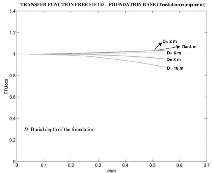
Figure 6. Transfer function of the translation component with the normalized frequency for the type 1 soil profile, width and length foundation 10 m, and burial depths of the foundation 2 m, 4 m, 6 m, 8 m y 10 m.
