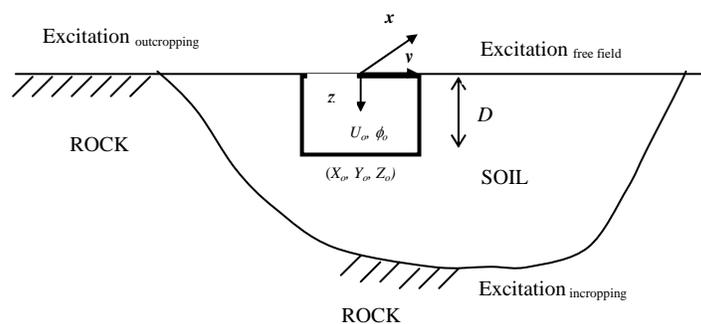
Figure 1. Configuration of rock, soil profile, foundation and possible location of the input ground motion for the kinematic interaction analysis.
