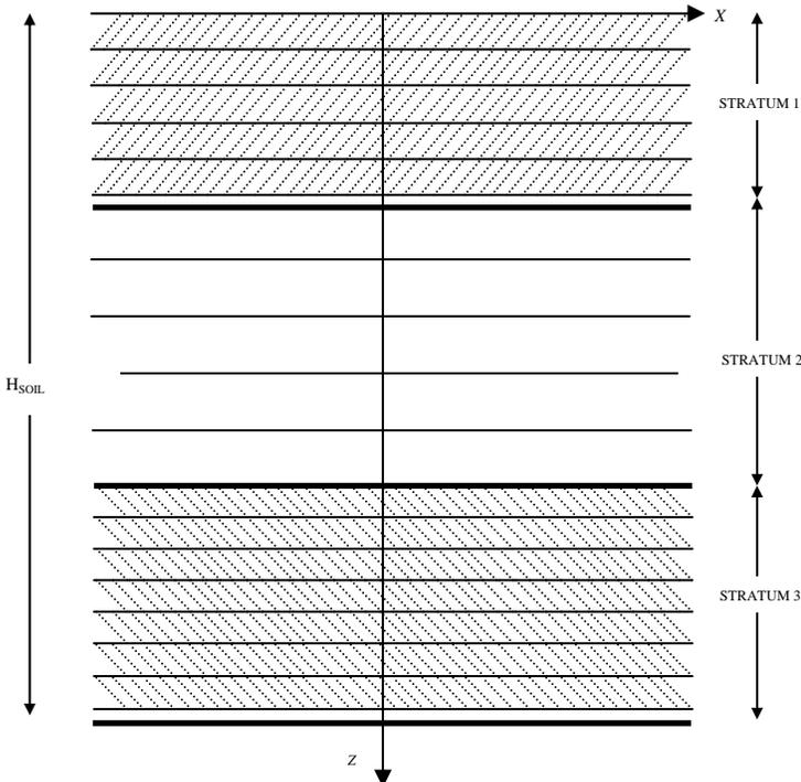
Figure 2. illustrative example of the division of a soil profile, composed by 3 strata, into 17 sub-strata.
