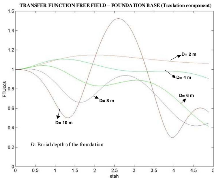
Figure 12. Transfer function of the translation component with the normalized frequency for the type 4 soil profile, width and length foundation 10 m, and burial depths of the foundation 2 m, 4 m, 6m, 8m y 10 m.
