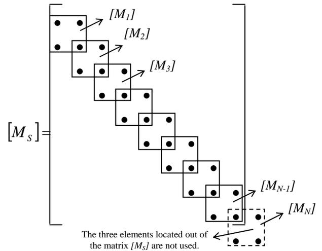
Figure 4. Assembly of the mass matrix of the soil profile  $[M_S]$ .
