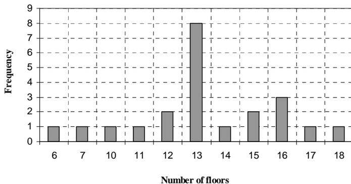
Figure 14. Frequency histogram of number of floors of damaged buildings in the city of Cali, by the earthquake of November 15, 2004.
