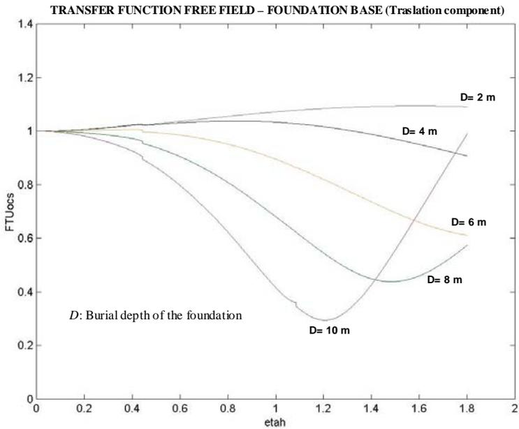
Figure 8. Transfer function of the translation component with the normalized frequency for the type 2 soil profile, width and length foundation 10 m, and burial depths of the foundation 2 m, 4 m, 6m, 8m y 10 m.
