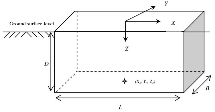
Figure 5. Variables of geometry and location of the reference point for the analysis of the effective earthquake excitation on the foundation base.
