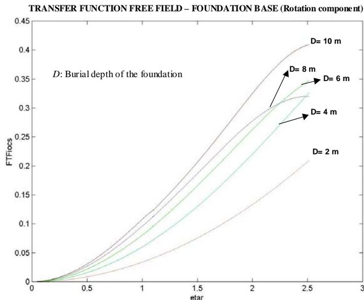
Figure 11. Transfer function of the rotation component with the normalized frequency for the type 3 soil profile, width and length foundation 10 m, and burial depths of the foundation 2 m, 4 m, 6m, 8m y 10 m.
