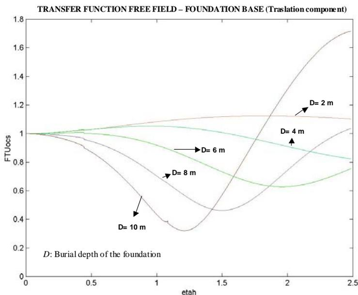
Figure 10. Transfer function of the translation component with the normalized frequency for the type 3 soil profile, width and length foundation 10 m, and burial depths of the foundation 2 m, 4 m, 6m, 8m y 10 m.
