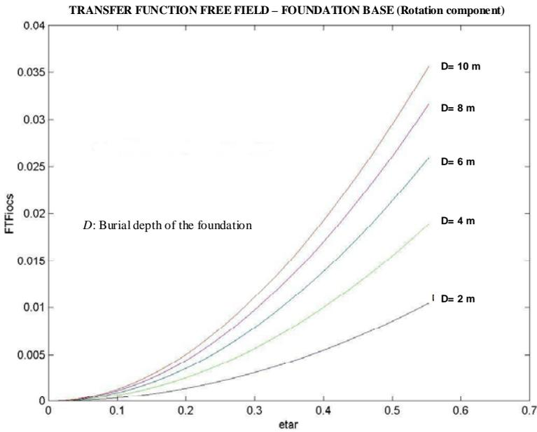
Figure 7. Transfer function of the rotation component with the normalized frequency for the type 1 soil profile, width and length foundation 10 m, and burial depths of the foundation 2 m, 4 m, 6m y 10 m.
