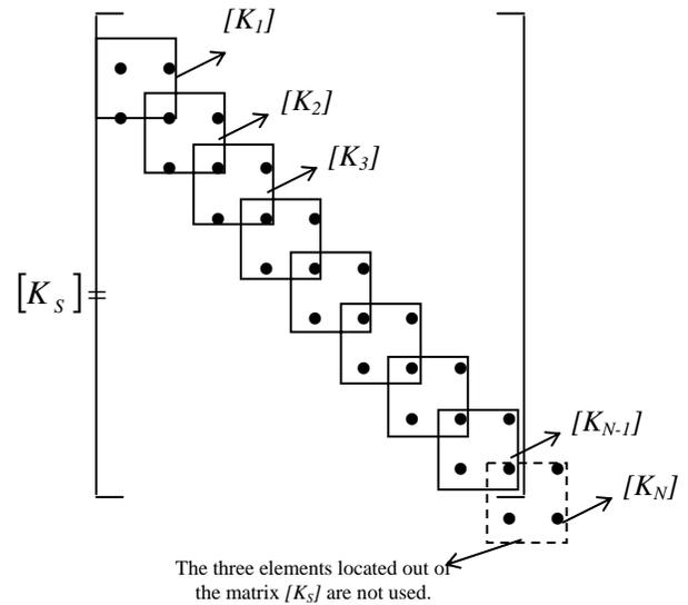
Figure 3. Assembly of the stiffness matrix of the soil profile  $[K_S]$ .
