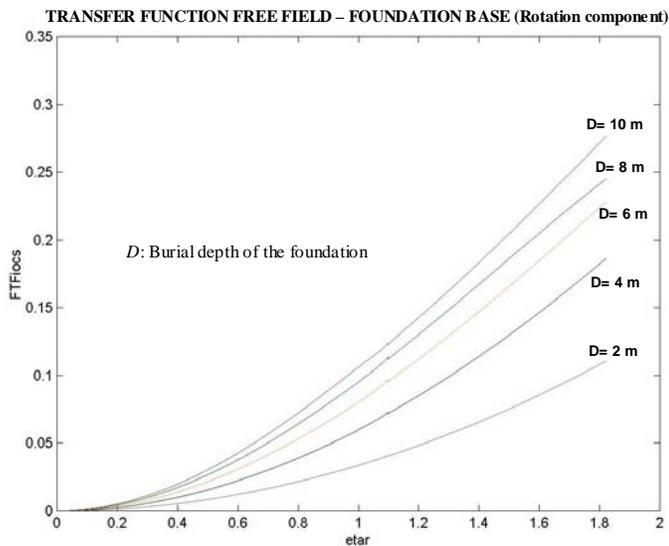
Figure 9. Transfer function of the rotation component with the normalized frequency for the type 2 soil profile, width and length foundation 10 m, and burial depths of the foundation 2 m, 4 m, 6m, 8m y 10 m.
