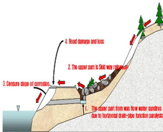
**Fig 15. Road breakage by the boulder flow**
