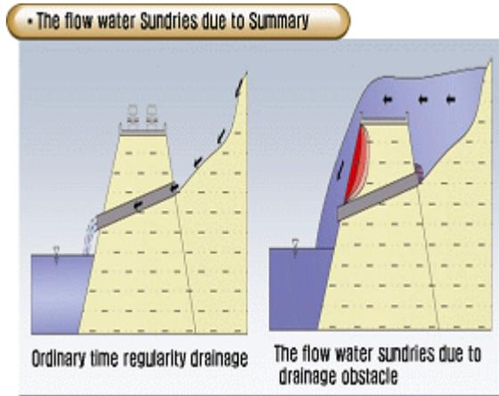
**Fig 13. Damage due to flow of extraneous material**
