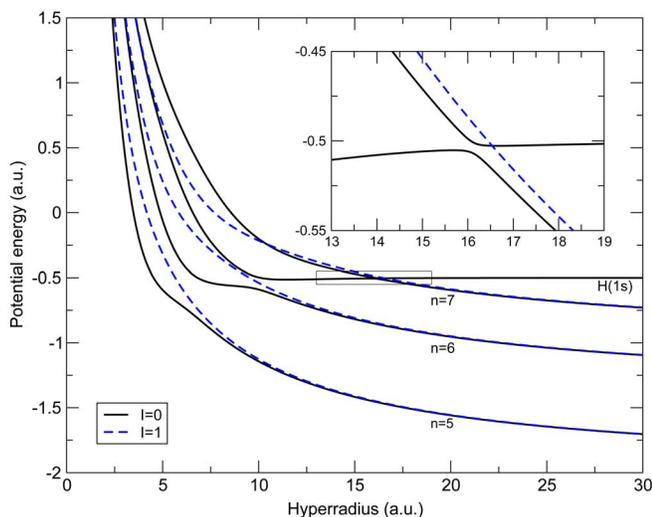
FIG. 2. (Color online) Selective seven diabatic potential energy curves of  $(\text{NeH})^{10+}$  used in the charge-transfer cross-section calculations. The solid lines are for  $l=0$  and dashed lines for  $l=1$ . The inset shows the avoided crossing between the  $\text{H}(1s)$  entrance channel and the first  $l=0$  channel from  $n=7$ .
