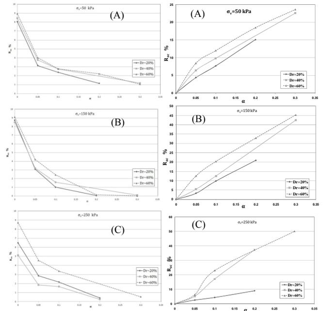
Fig. 10. Variation of  $(R_{ex})_{L10}$  due to Initial Static Shear Stress Ratio ( $\alpha$ ) for various values of Relative Density ( $D_r$ ) and Initial Normal Stress ( $\sigma_{v0}$ ) of: A) 10 kPa, B) 12 kPa, C) 15 kPa
