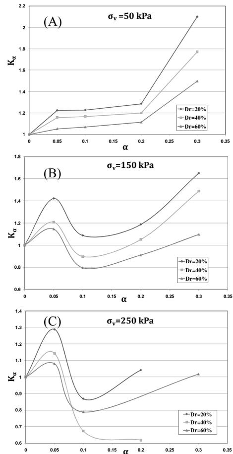
Fig. 8. Variation of  $K_\alpha$  due to Initial Static Shear Stress Ratio ( $\alpha$ ) for various values of Relative Density ( $D_r$ ) and Initial Normal Stress ( $\sigma_{v0}$ ) of; A) 50 kPa, B) 150 kPa, and C) 250 kPa
