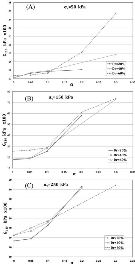
Fig. 9. Variation of  $(G)_{L10}$  due to Initial Static Shear Stress Ratio ( $\alpha$ ) for various values of Relative Density ( $D_r$ ) and Initial Normal Stress ( $\sigma_{v0}$ ) of: A) 10 kPa, B) 12 kPa, C) 15 kPa
