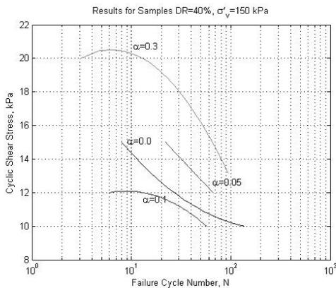
Fig. 7. Variation of Failure Cycle Number ( $N_f$ ) with cyclic shear stress amplitude (CSS) for test with Initial Normal Stress of 150 kPa and Relative Density of 40% and various Initial Static Shear Stress Ratio ( $\alpha$ )
