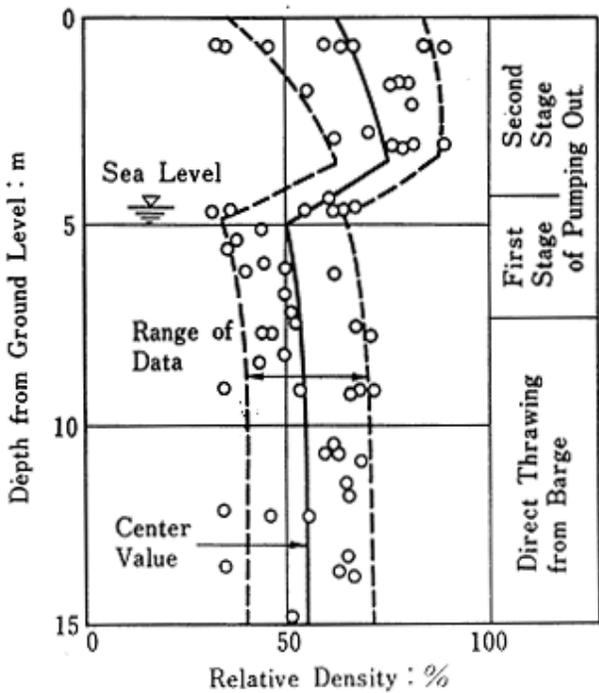
Fig. 9 Distribution of relative density of fill sand with depth (after Ad Hoc Com. 1977)
