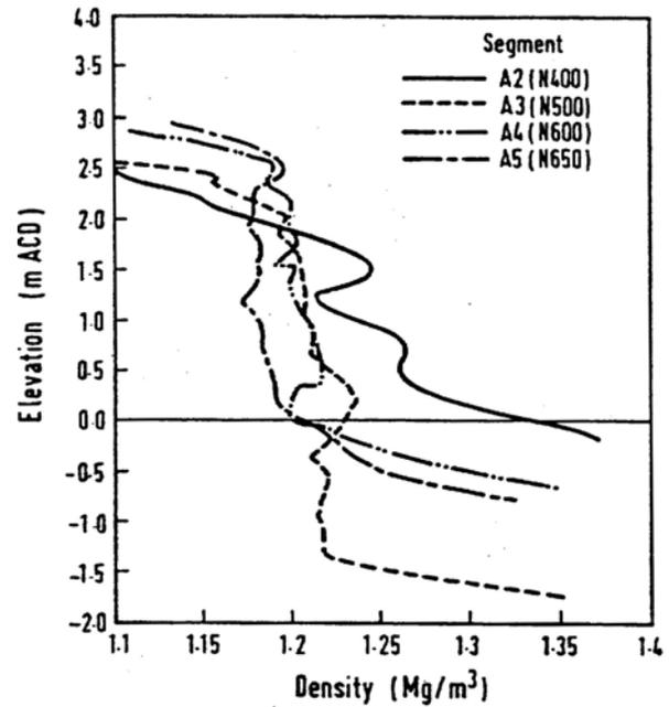
Fig. 7 Density of clay in A2 to A5
