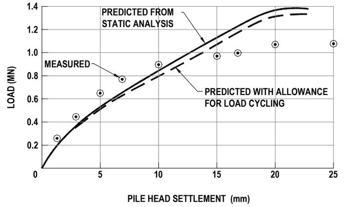
Fig. 13. Predicted load-settlement behaviour for pile head.
