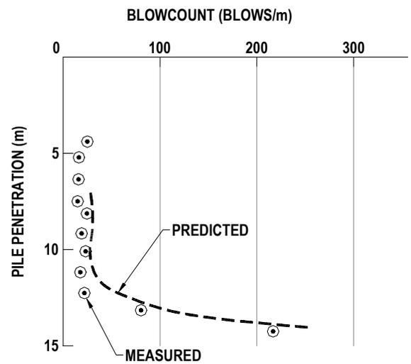
Fig. 14. Predicted blowcount during driving.
