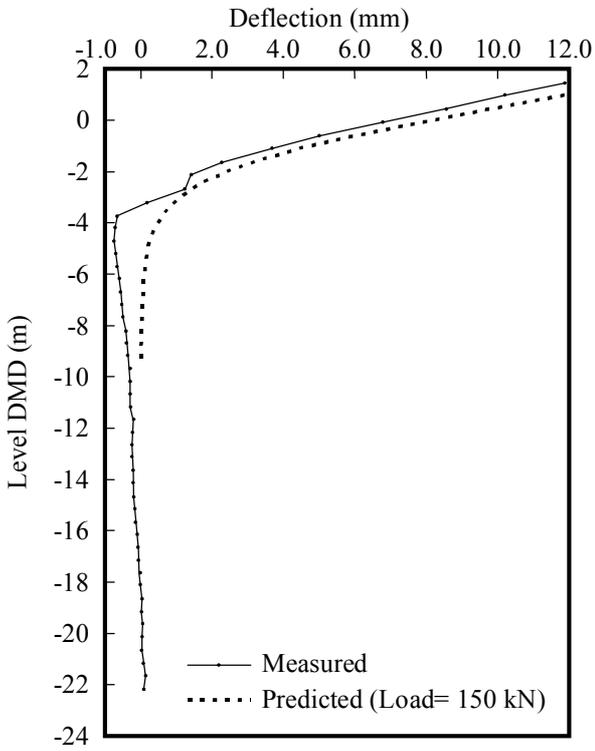
Fig. 11. Measured and predicted deflection distributions – pile P2(H).
