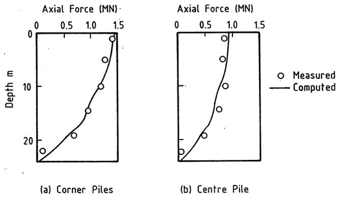
Fig. 16. Measured and computed load distributions along piles.
