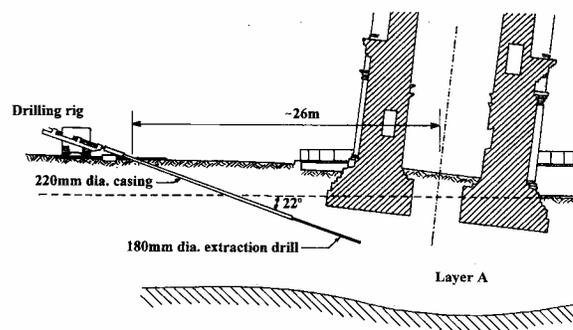
Fig. 10. Concept of soil extraction alongside and beneath the Tower
