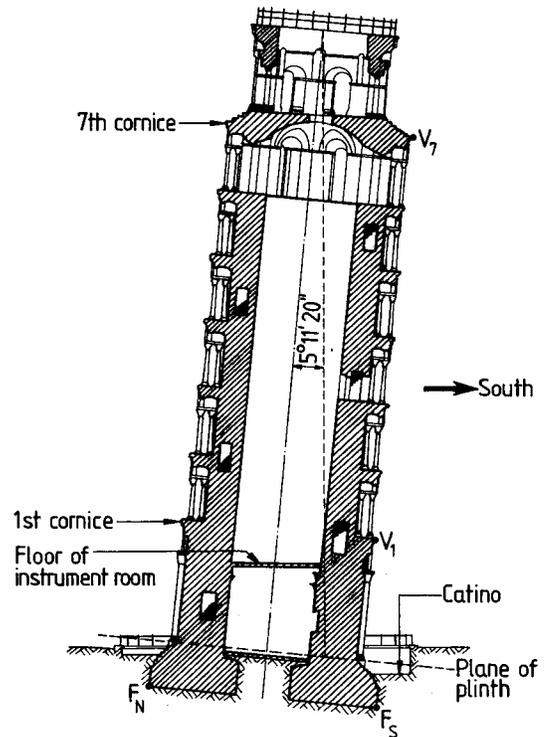
Fig. 2. Cross-section through the Leaning Tower of Pisa
