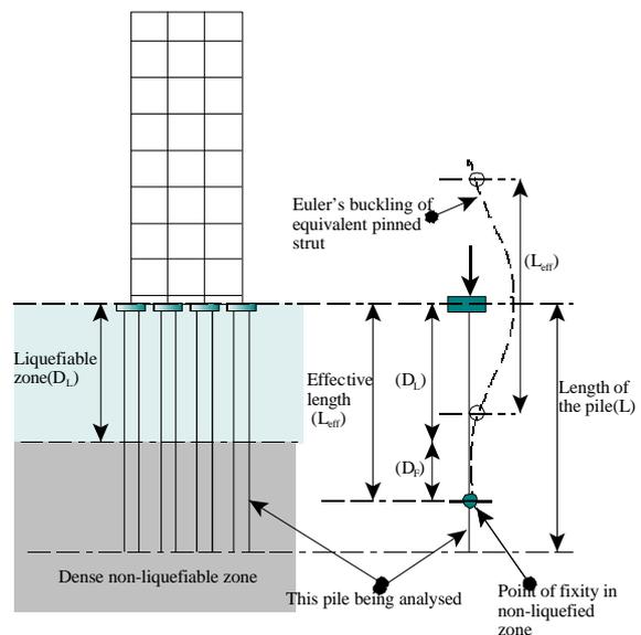
Figure 11: Idealisation of buckling instability of piled foundation.
