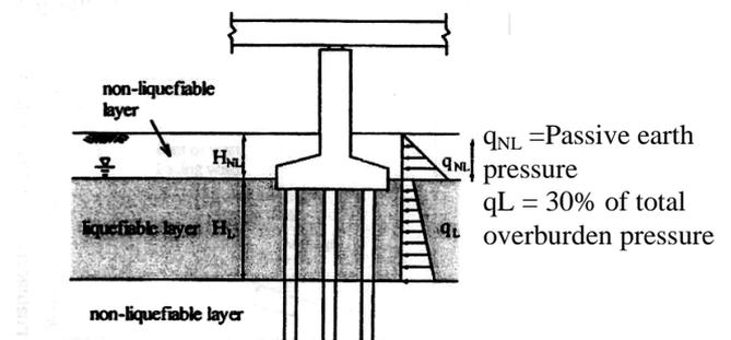
Fig 1. JRA (1996) code of practice showing the idealization for seismic design of bridge foundation.
