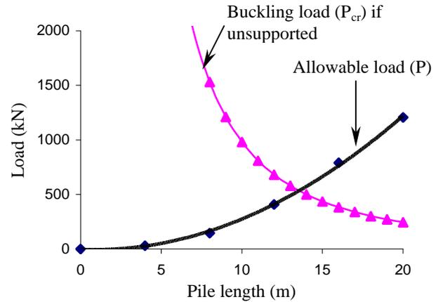
Figure 4: Allowable load and buckling load of a typical pile (if unsupported).
