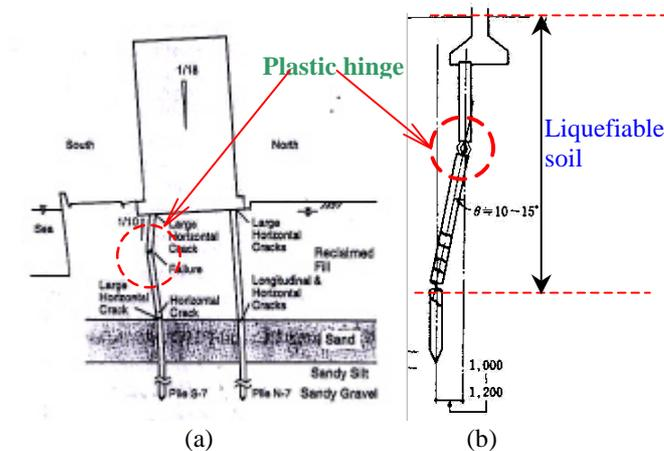
Figure 3: Failure of piled buildings; (a) A collapsed building after the 1995 Kobe earthquake, showing the hinge formation after Tokimatsu et al. (1997); (b): Failure piles of the NHK building after Hamada (1992b).
