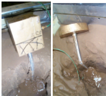
Figure 8: Some failed piles in the centrifuge tests. The tests were carried out in level grounds to avoid lateral spreading.
