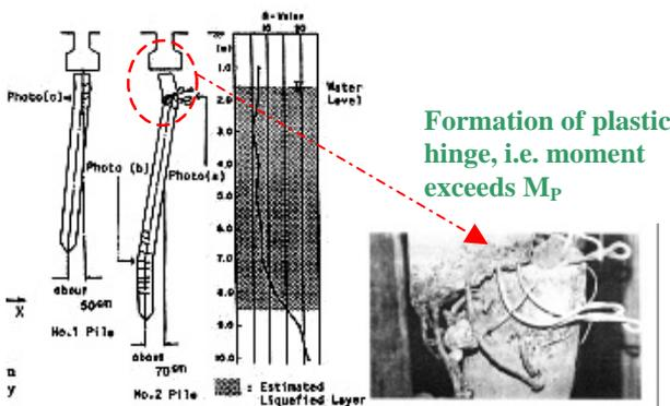
Figure 2: Failure of piles in NFCH building during the 1964 Niigata earthquake, Hamada (1992a).
