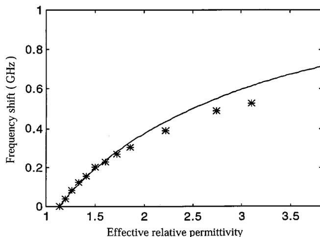
Fig. 8. Measured (\*) and calculated (solid line) values of the frequency shift as a function of the effective relative permittivity.
