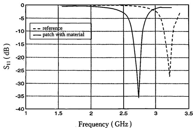
Fig. 2. The  $S_{11}$  characteristics of a patch source with (dark curve) and without (light curve) thermal gasket material.
