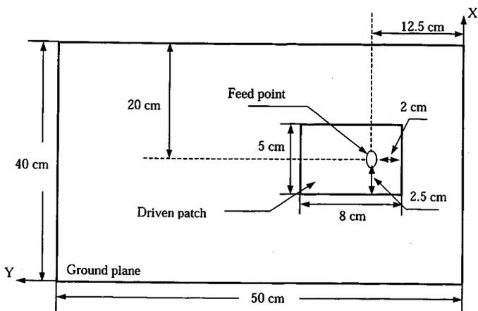
Fig. 7. Driven-patch dimensions for exciting the  $TM_{010}^z$  mode.
