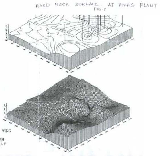
Figure 3 Hard Rock Surface at Visakhapatnam Plant
