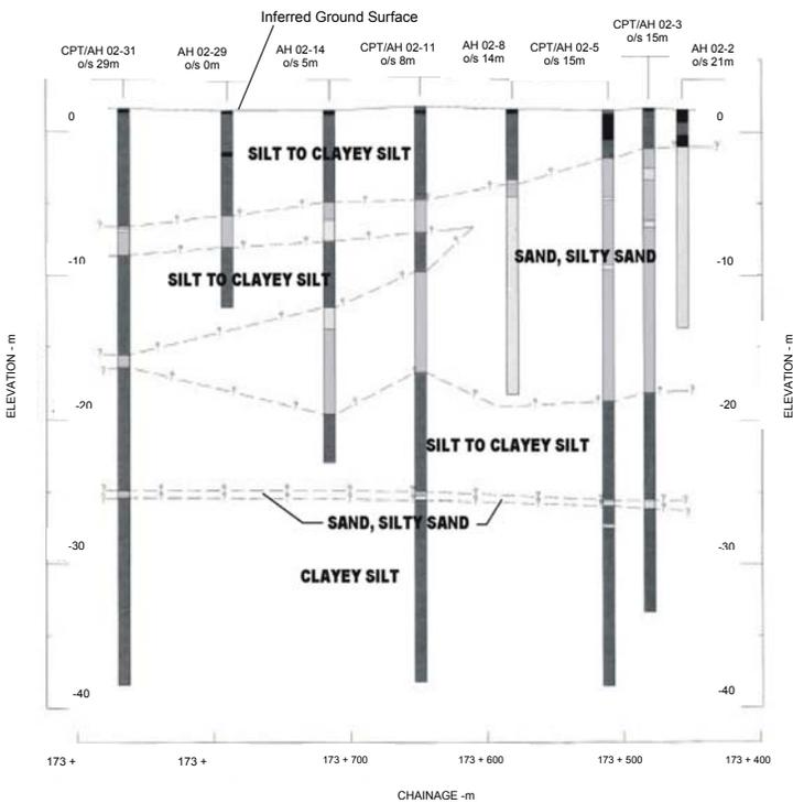
Fig. 2 Inferred soil conditions (from west to east).
