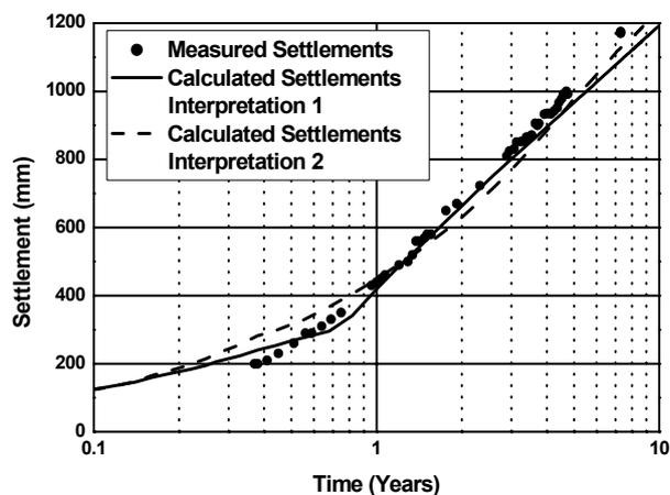
Fig. 7 Measured and Calculated Ground Settlements
