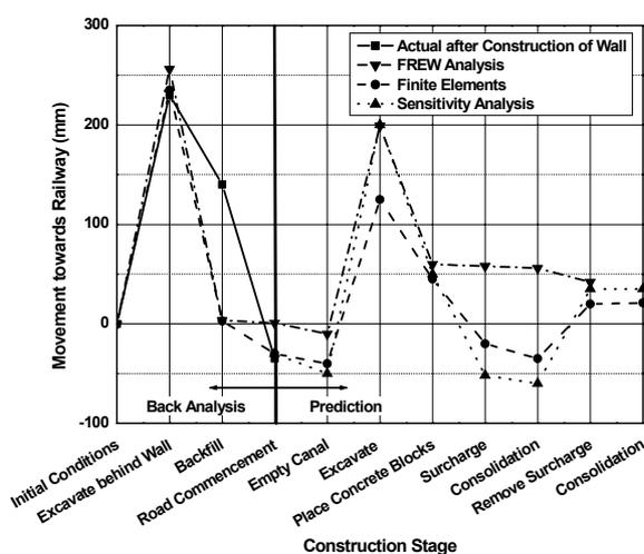
Fig. 5 Horizontal Wall Movements Calculated using FREW & SAFE
