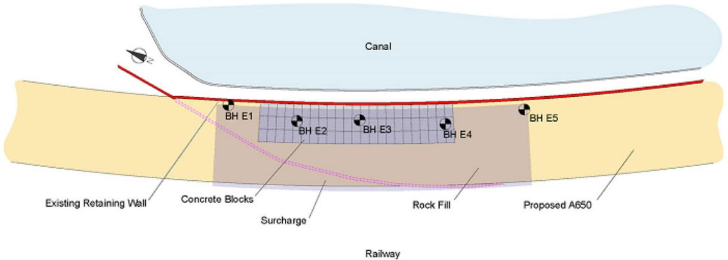
Fig. 2 Schematic plan of special earthworks, borehole location, canal wall and canal
