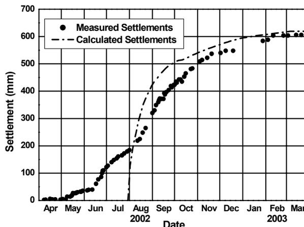
Fig. 9 Settlements behind Wall during Surcharge Placement
