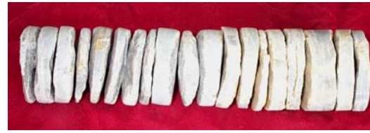
Fig. 1. Rock disk produced in drilling
