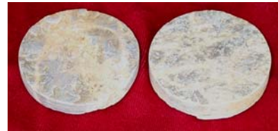
Fig. 2. Rock-core disked morphology
