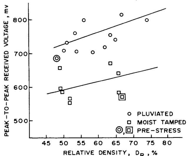
Figure 3. Signal Attenuation Versus Relative Density, Dover 40-50 Sand
