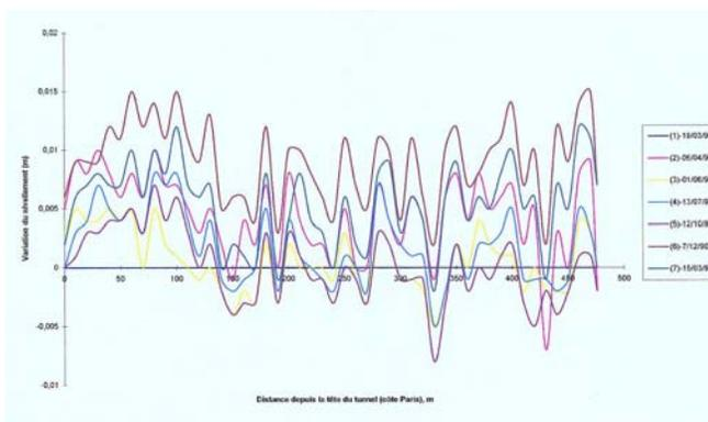
Fig. 5. Leveling defects (track 1, rail 1)
