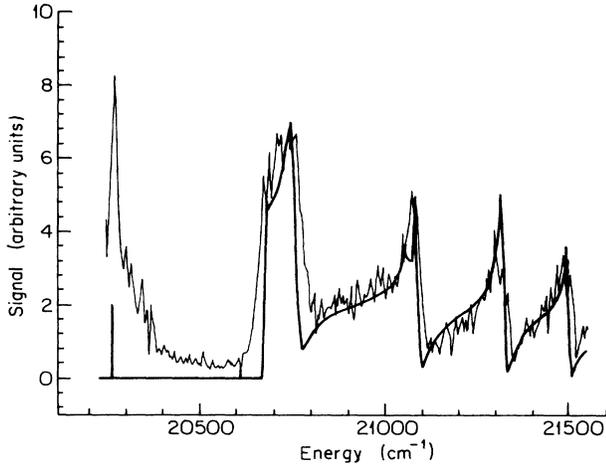
FIG. 3. Shake-off spectrum obtained from exciting the transition,  $\text{Ba}(6s19d) \rightarrow \text{Ba}^+(6p_{1/2}) + e^-$ , by detecting the fluorescence from the excited  $\text{Ba}^+(6p_{1/2})$  ions. The resonances are  $\text{Ba}(6p_{3/2}nd)$  states with  $11 \leq n \leq 14$ .
