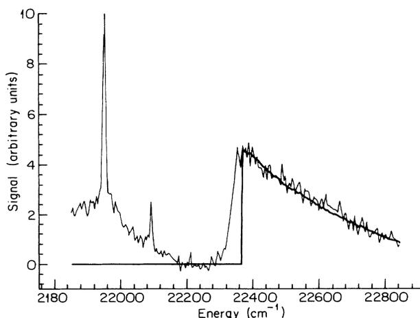
FIG. 2. Shake-off spectrum obtained from exciting the transition,  $\text{Ba}(6s19d) \rightarrow \text{Ba}^+(6p_{3/2}) + e^-$ , by detecting the fluorescence from the excited  $\text{Ba}^+(6p_{3/2})$  ions.
