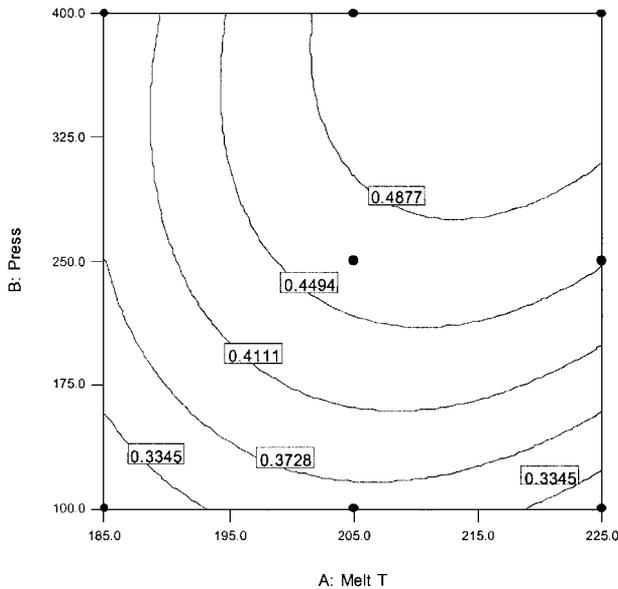
**3** Predicted shrinkage from mould for small metal injection molded part: contours show green part dimensions as percentage of mould dimensions. Note region of low variability (widely spaced contour lines) at high transfer pressure (bar) and high feedstock melt temperature (celsius)
