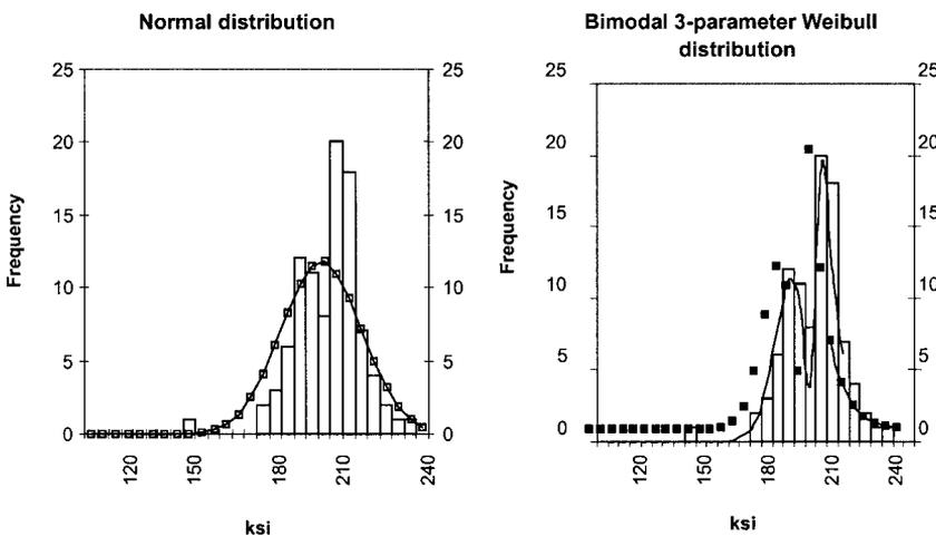
**4** Histograms of transverse rupture strength data from single batch of 96 pressed and sintered FL-4605 steel test bars. Compared with Gaussian distribution (left) most often used to represent mechanical properties data, bimodal three-parameter Weibull distribution (right) shows excellent fit
