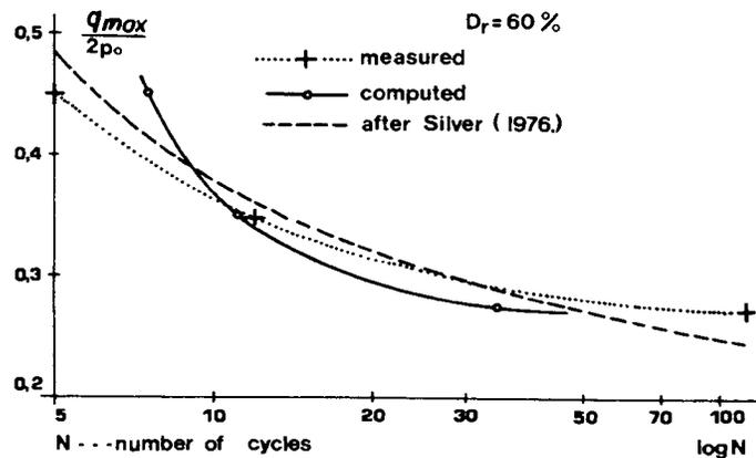
Fig.5. Computed and measured numbers of cycles to liquefaction
