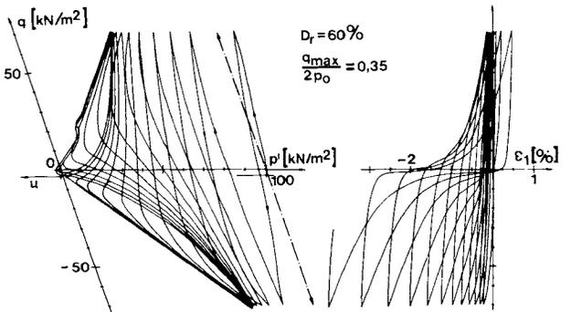
Fig. 3. Effective stress paths and stress-strain curves for two different cyclic stress ratios
