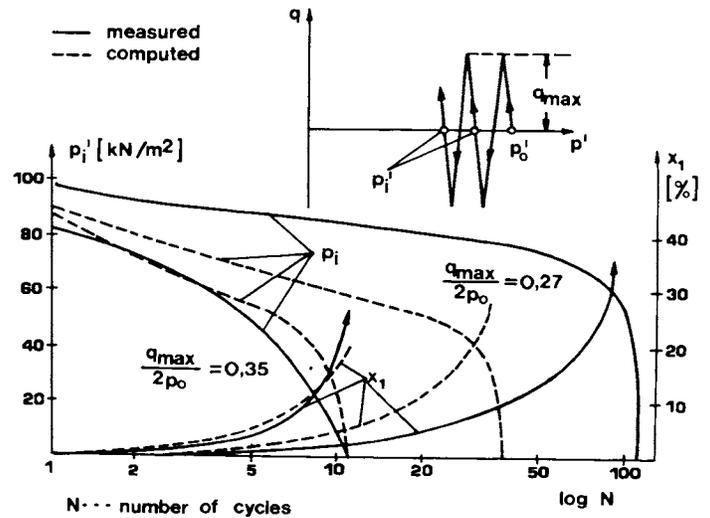
Fig.6. Computed and measured values of x<sub>1</sub> and p<sub>i</sub> for two characteristic tests
