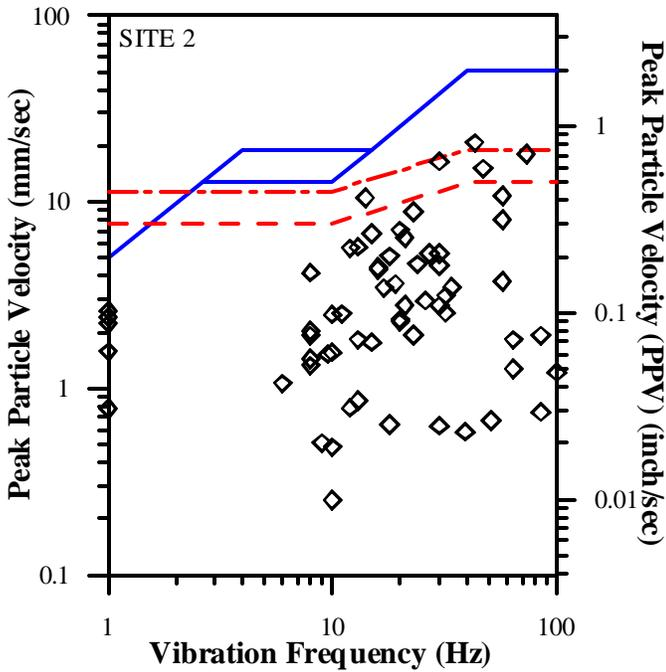
Fig. 6. PPV vs. Vibration Frequency for Site 2.
