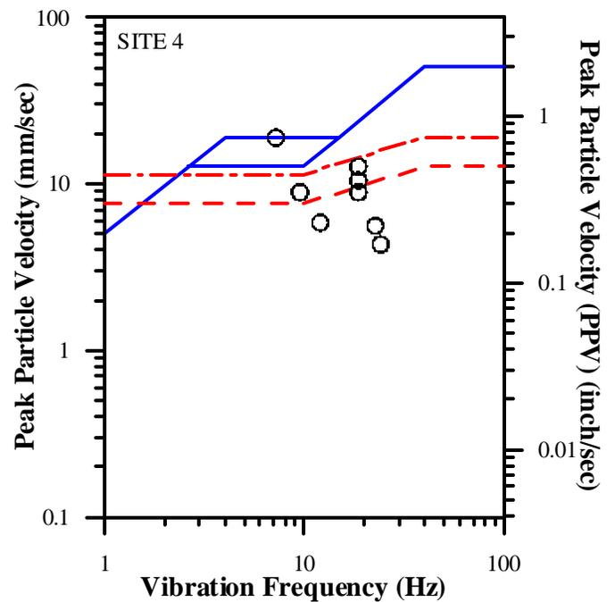
Fig. 8. PPV vs. Vibration Frequency for Site 4.
