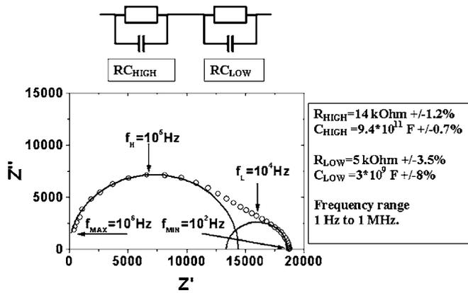
FIG. 3. Impedance spectra of 5% SrTiO<sub>3</sub> slurry in butoxyethanol: open circles represent experimental data, and lines represent fitting by two ideal RC circuits [ $R_H=14\text{ k}\Omega(\pm 1\%)$ ;  $C_H=0.94\times 10^{-10}\text{ F}(\pm 0.7\%)$ ;  $R_L=5\text{ k}\Omega(\pm 3\%)$ ;  $C_L=3\times 10^{-9}\text{ F}(\pm 8\%)$ ].
