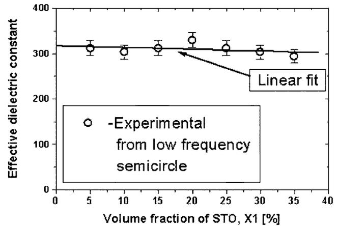
FIG. 4. Effective dielectric constant of SrTiO<sub>3</sub> particles (in butoxyethanol) determined from low frequency semicircle in Fig. 3 as a function of solid loading in slurries. Error bars correspond to standard deviation of effective dielectric constant  $\Delta=5\%$ .
