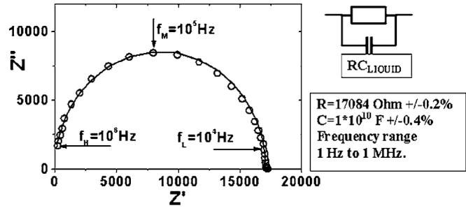
FIG. 2. Impedance spectra of butoxyethanol; open circles represent experimental data, and line represents fitting with an ideal RC circuit [ $R = 17 \text{ k}\Omega (\pm 0.2\%)$ ;  $C = 1 \times 10^{-10} \text{ F} (\pm 0.4\%)$ ].
