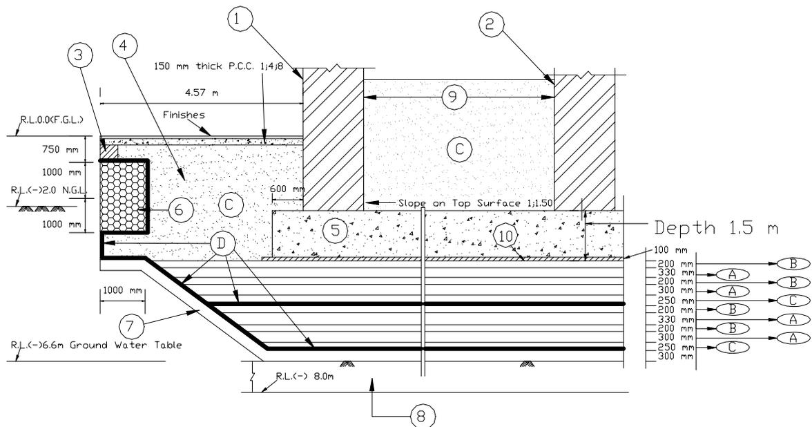
(A) Boulders (size not less than 175mm) with smaller in filling stones and quarry spoil/stone screening rolled with 10 T roller eight times, (B) Boulders (size 90mm – 40mm) with smaller in filling stones and quarry spoil/stone screening rolled with 10 T roller eight times, (C) Compacted sand, (D) Geocomposite comprising of rope mattress and geofilter
