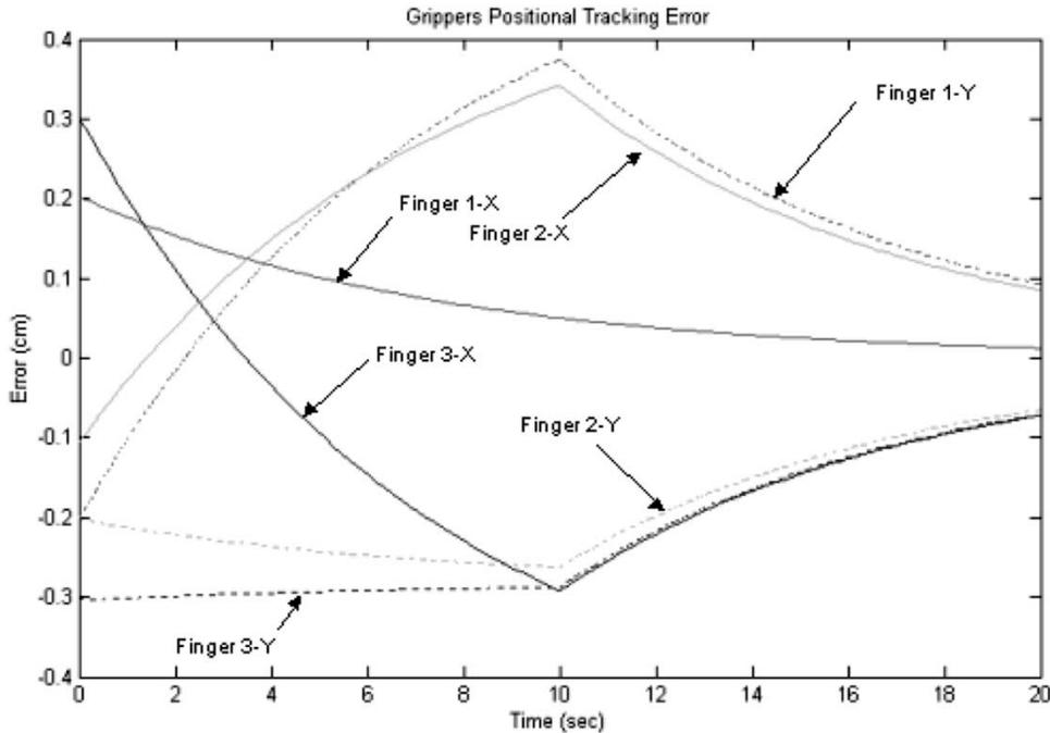
Fig. 6. Tracking errors using PD object contact controller.
