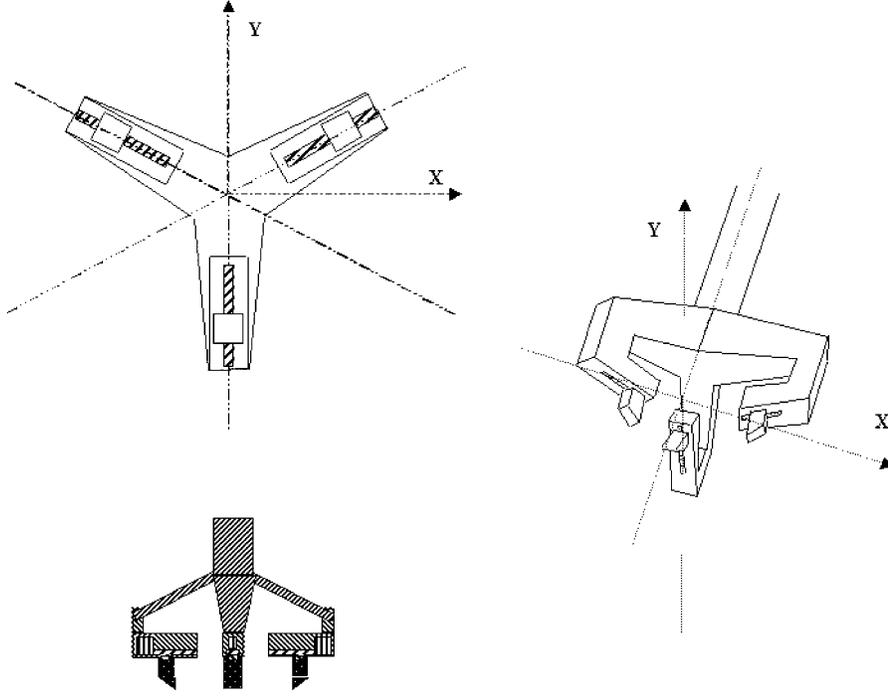
Fig. 1. Schematic of a three-finger robot gripper.
