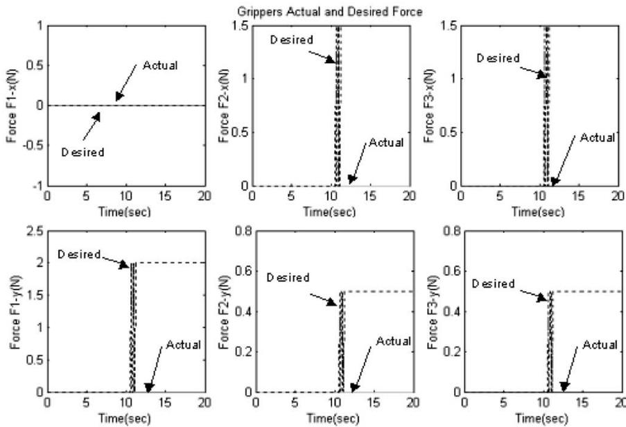
Fig. 8. Force response without the adaptive NN critic.
