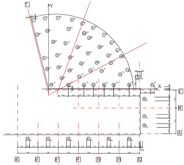
Fig. 5 Pile drawing for the extension of the building "C2"
