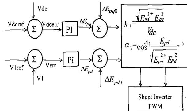
Fig. 2 Shunt branch control of the UPFC.
