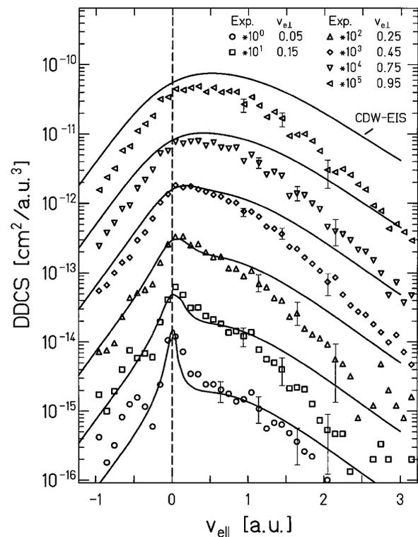
FIG. 1. Doubly differential cross sections  $\text{DDCS} = d^2\sigma / (dv_{\parallel} dv_{\perp} 2\pi v_{\perp})$  as functions of the longitudinal electron velocity for certain transverse velocity cuts in pure singly ionizing 3.6 MeV/u  $\text{Au}^{53+}$  on Ne collisions. DDCS at different  $v_{\perp}$  are multiplied by factors of 10, respectively. Lines: theoretical CDW-EIS results.
