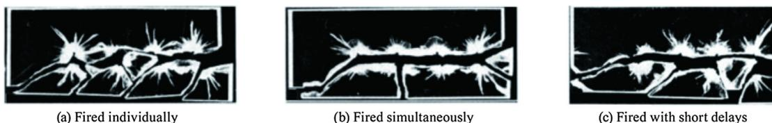
Fig. 4. Effects of using delays on presplit holes [10].
