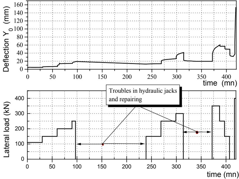
Fig. 3. Load-deflection evolution in loading tests
