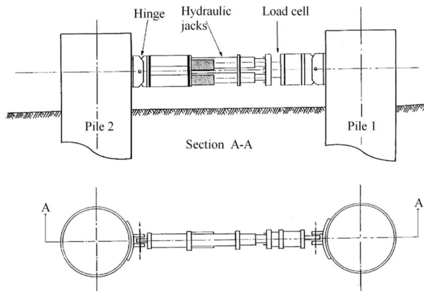
Fig. 2. Schematic experimental set-up of pile loading (Pouget, 1988)
