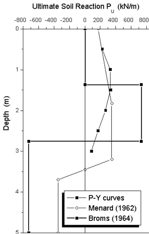
Fig. 10. Profiles of ultimate soil reaction.
