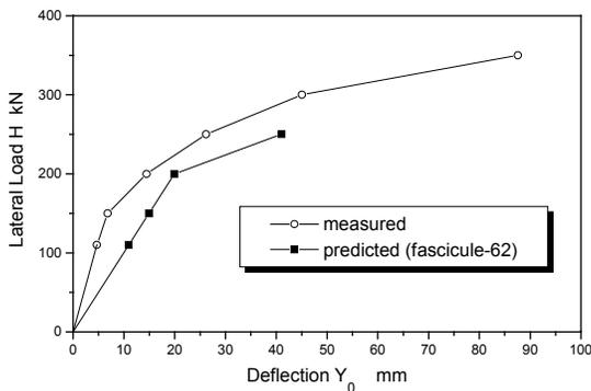
Fig. 6. Load-deflection curve of pile 1.
