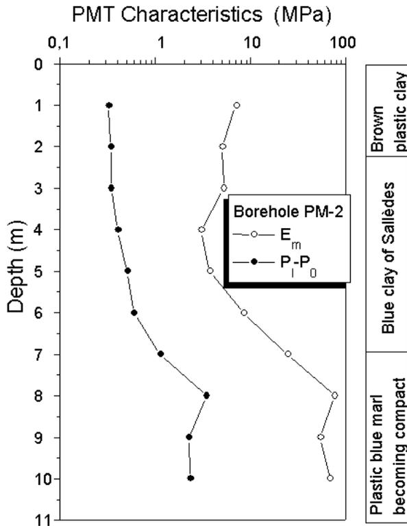
Fig. 1. Typical PMT characteristics of the site Salledes
