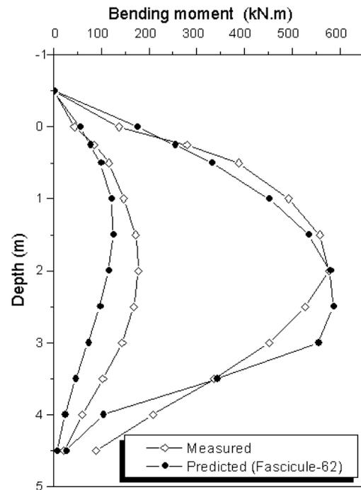
Figure 11. Predicted and measured bending moments.
