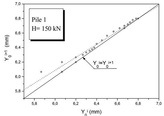
Fig. 4. Evolution of pile deflection for a load of 150 kN
