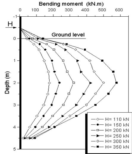
Fig. 7. Bending moment profiles of pile 1.
