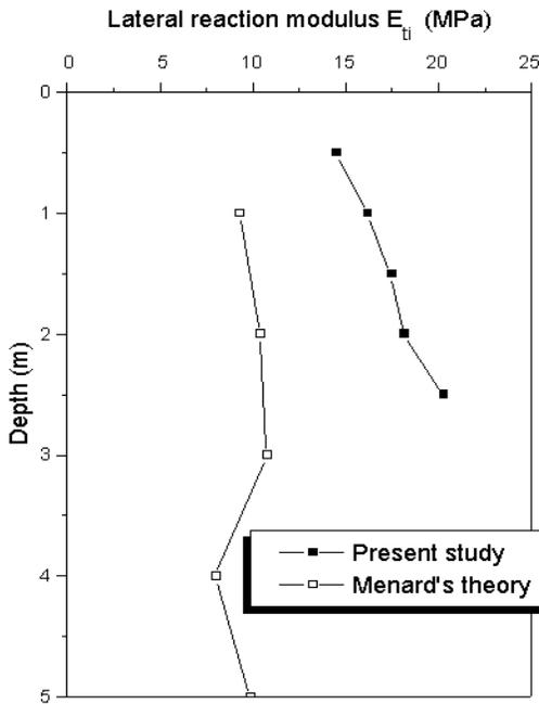
Figure 9. profiles of lateral reaction modulus
