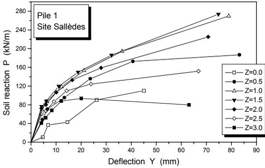
Fig. 8. P-Y curves of pile 1.
