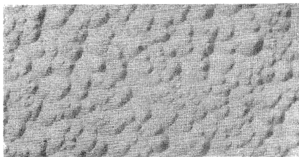
Figure 2. (100) surface morphology of InP grown with \text{PCl}_3 . White bar is 500\mu\text{m} long
