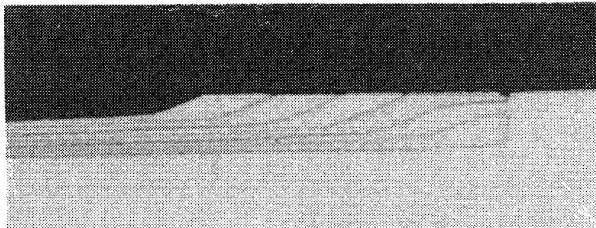
Figure 5. Regrowth of alternating p- and n-type InP around 5.4 \mu\text{m} high mesas with 6 \times 10^{-6} moles \text{min}^{-1} \text{PCl}_3 .
