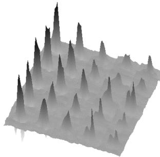
**FIGURE 4.** A microwave image of an array of pittings at 67 GHz.
