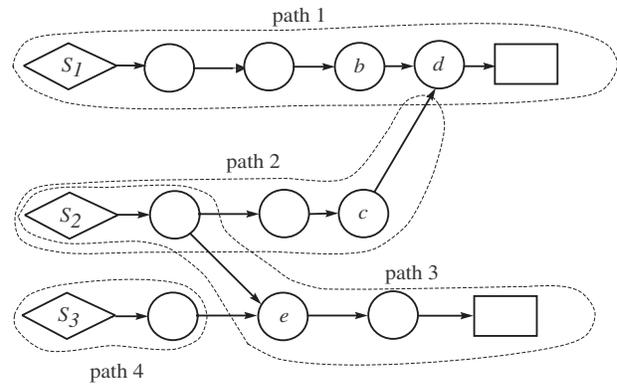
**Figure 1. The DAG model for the applications (circles) and data transfers (arrows). The diamonds and rectangles denote sensors and actuators, respectively. The dashed lines enclose each path formed by the applications.**
