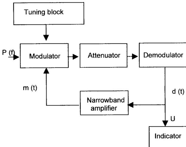
Fig. 4. Scheme of automodulation measuring system.
