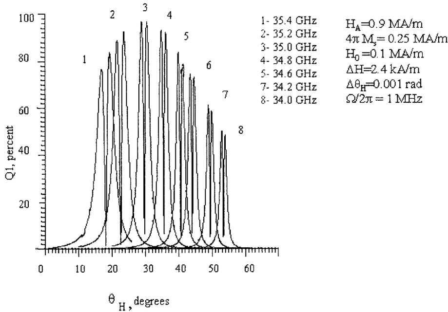
Fig. 2. Amplitude of the first harmonic of modulation frequency versus the HFR angle of orientation.
