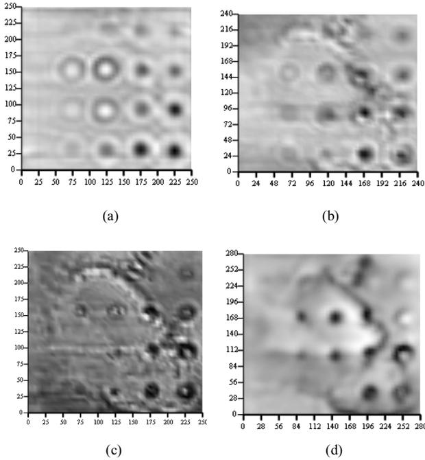
Figure 3: Millimeter wave image of panel A1 at different frequencies (dimensions are in mm): (a)  $f = 33.5$  GHz with a horn antenna; (b)  $f = 70$  GHz with a horn antenna; (c)  $f = 100$  GHz with a horn antenna; (d)  $f = 100$  GHz with a lens antenna.
