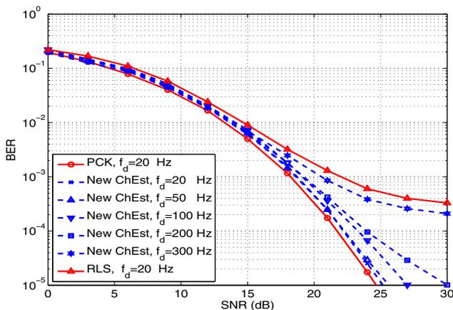
Fig. 6. BER versus SNR of a single-antenna receiver.
