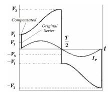
Fig. 5 (b) Voltage levels in original series voltage inverting method and in voltage compensation method.
