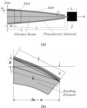
Fig. 7 (a)Tapered beam and its (b)bending element.
