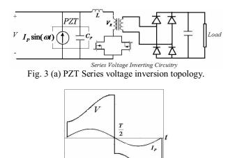
Fig. 3 (b) PZT voltage and current waveforms
