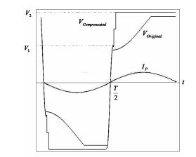
Fig. 4 (b) Voltage waveforms in original parallel voltage inverting method and in voltage compensation method with two-step compensation.
