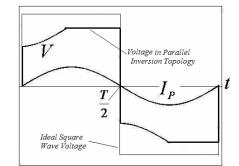
Fig. 2 (b) PZT voltage and current waveforms.
