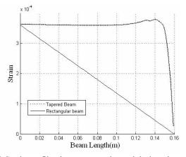
Fig. 9 Strain profile along rectangular and designed tapered beam.
