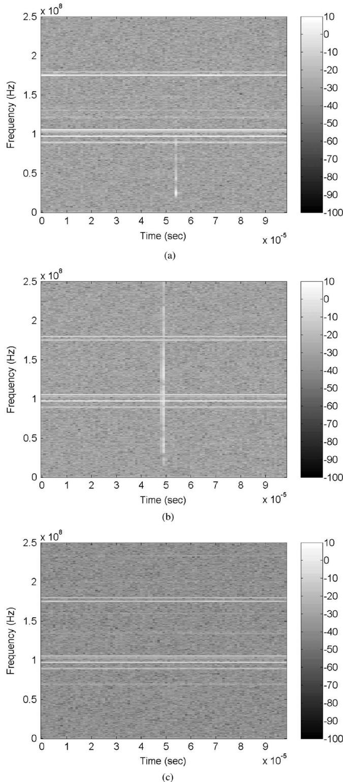
Fig. 4. Spectrogram of ambient noise and of emissions from different automobiles when a spark event was captured. (a) Emissions from vehicle “A” during a spark event. (b) Emissions from vehicle “B” during a spark event. (c) Ambient noise (reference).
