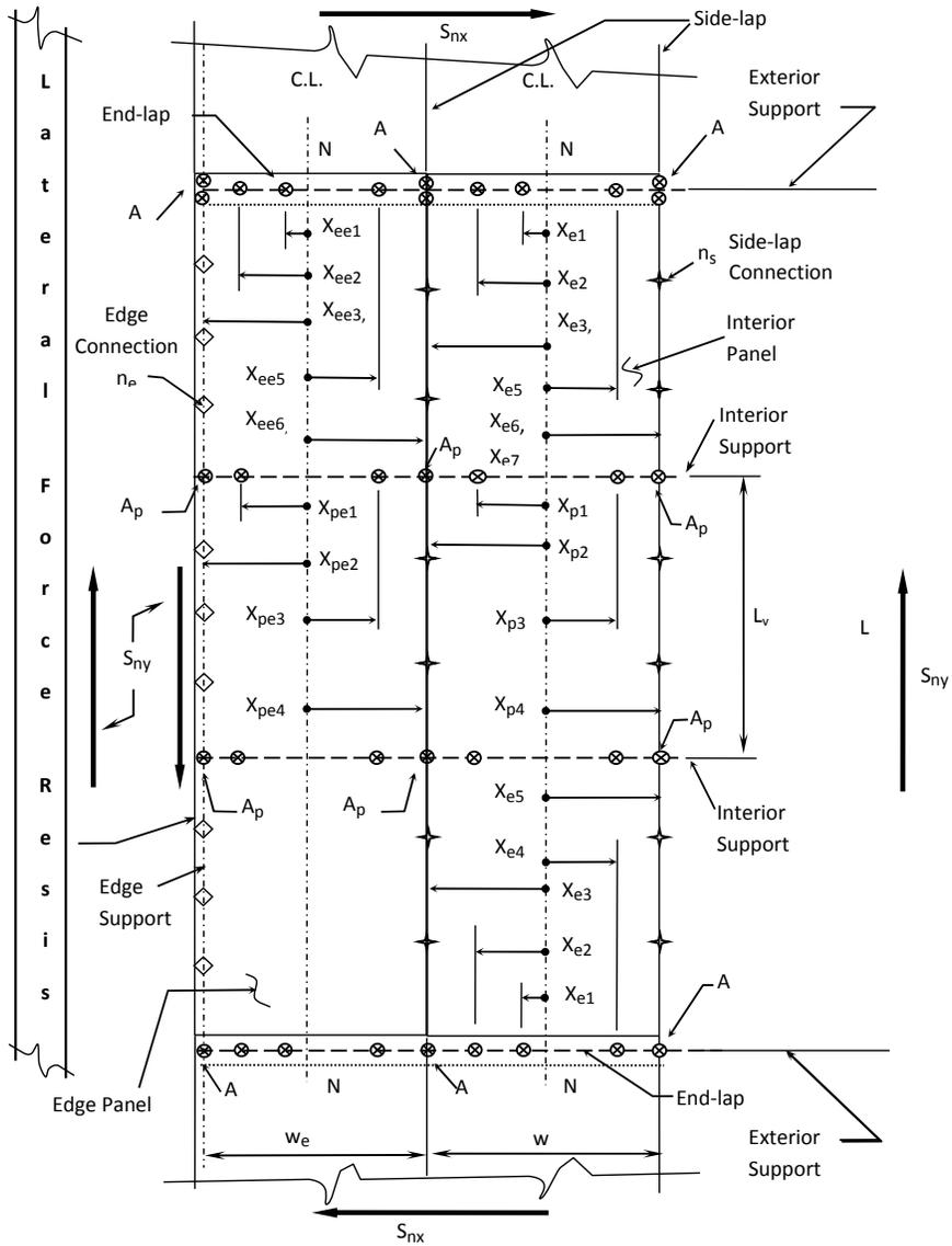
Figure 1 Schematic Illustration of Section 3a Parameters
