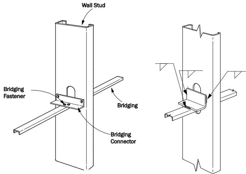
**Figure 1 - Examples of Bridging Connector Assemblies**
