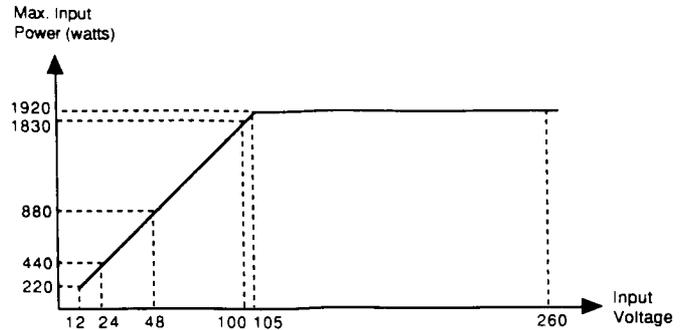
Fig. 4. Maximum Permissible Input Power vs Input Voltage.
