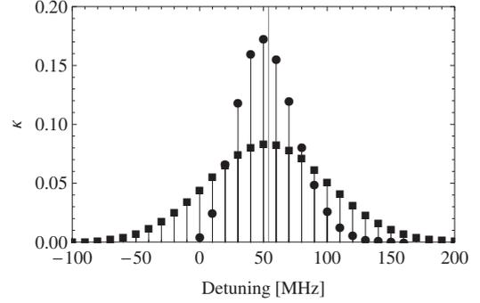
FIG. 6. Sideband spectrum of a collinearly excited  $\text{He}^+$  ion with a secular frequency of  $\omega_s = 2\pi \times 10 \text{ MHz}$ . The vertical line indicates the recoil frequency of 54 MHz. Circles and squares indicate whether the ion is assumed to be cooled to the ground state of motion or to 1 mK, respectively.
