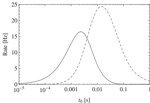
FIG. 3. Optimization of the interaction time  $t_0$  with the exciting laser field to maximize either the excitation rate (solid line) or the resonant three-photon ionization rate (dashed line). The dead time is set to zero and the laser intensity is assumed to be  $10 \mu\text{W}/\mu\text{m}^2$ .
