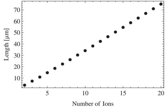
FIG. 5. Numerically determined length  $l_i$  of an  $\text{He}^+$  ion chain with constant radial confinement of  $\omega_r = 2\pi \times 10$  MHz and variable axial confinement to maintain a linear string. The length is well approximated linearly by  $l_i \sim N 4 \mu\text{m} - 5 \mu\text{m}$ .
