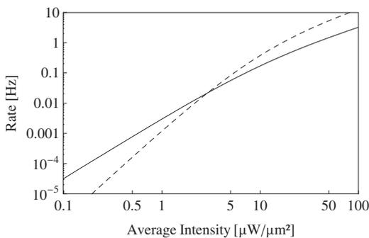
FIG. 11. Maximum excitation (solid line) and ionization rates (dashed line) for one collinearly excited  $\text{He}^+$  ion. The Rabi frequency has been reduced to 10%. Since the ionization cross section remains unchanged, the dynamics is slightly different from that in Fig. 4.
