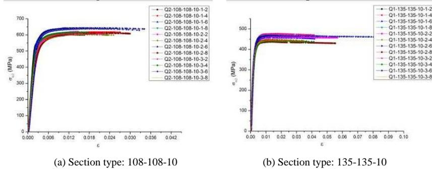
Fig. 10 Typical stress-strain curves for corner coupons
