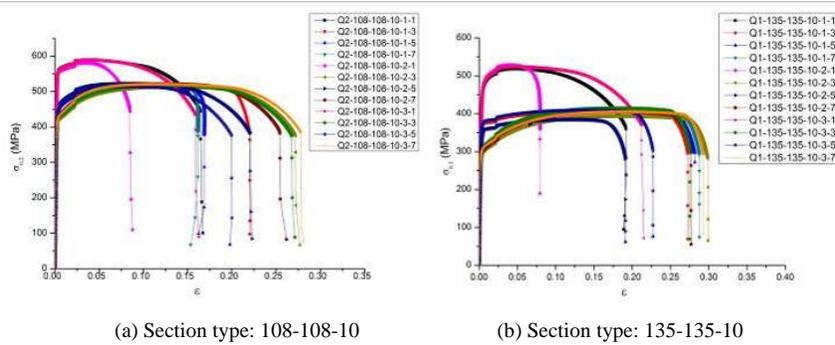
Fig.8 Typical stress-strain curves for flat coupons
