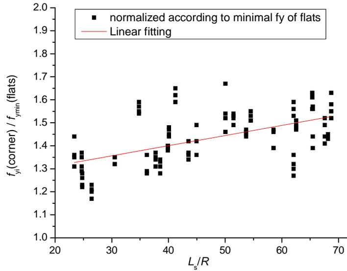
Fig. 15 Increase of yield strength versus  $L_s/R$  ratios for corner coupons
