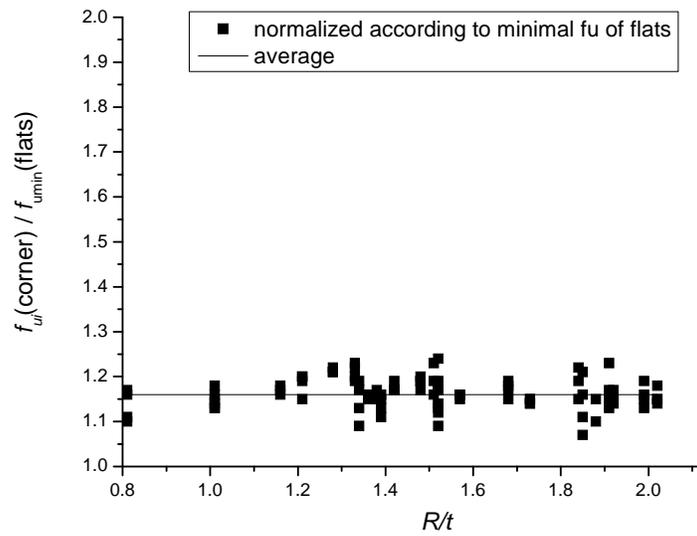
Fig. 16 Increase of ultimate strength versus  $R/t$  ratios for corner coupons
