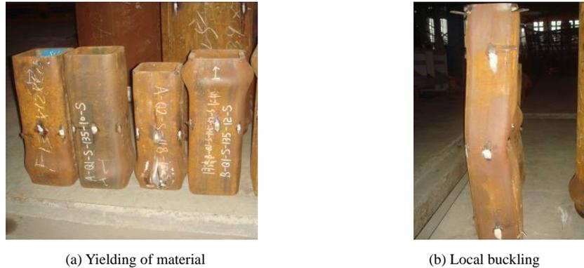
Fig. 12 Typical failure modes of stub columns
