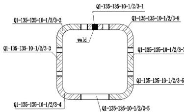
Fig. 5 Numbering of coupons for section 135-135-10
