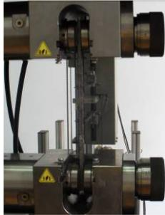
Fig. 3 Test set-up for flat and rounded coupons
