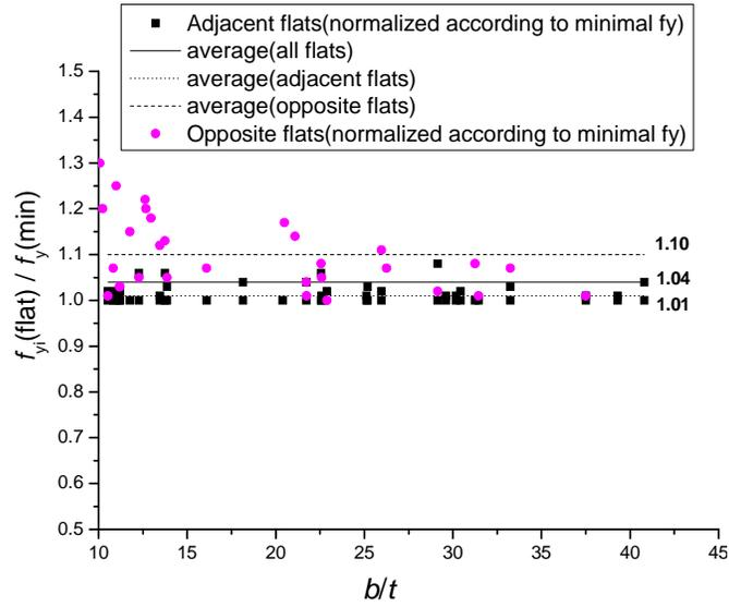
Fig. 13 Effect of  $b/t$  ratios for flat coupons
