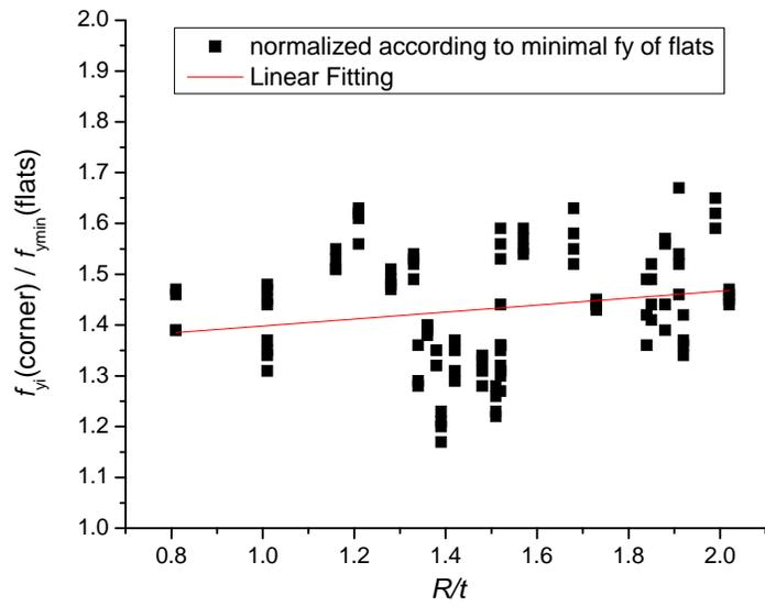
Fig. 14 Increase of yield strength versus  $R/t$  ratios for corner coupons
