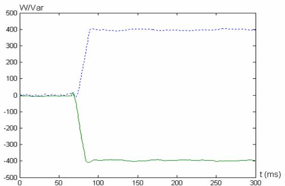
Fig. 10: Experimental PQ step change from (0,0) to (400,-400)
