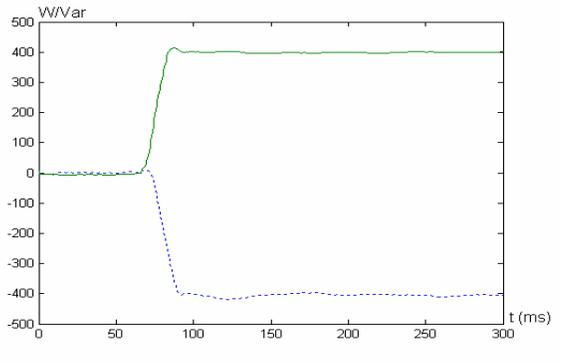
Fig. 11: Experimental PQ step change from (0,0) to (-400,400)
