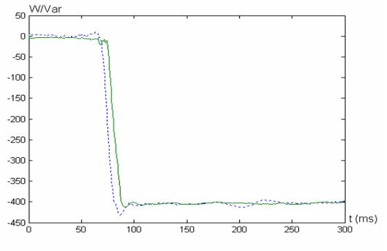
Fig. 12: Experimental PQ step change from (0,0) to (-400,-400)
