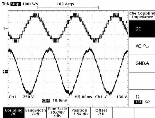
Fig. 8: Inverter line-line voltage and line current (5A/div)
