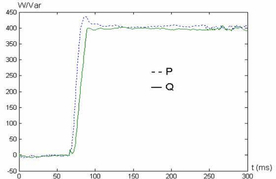
Fig. 9: Experimental PQ step change from (0,0) to (400,400)
