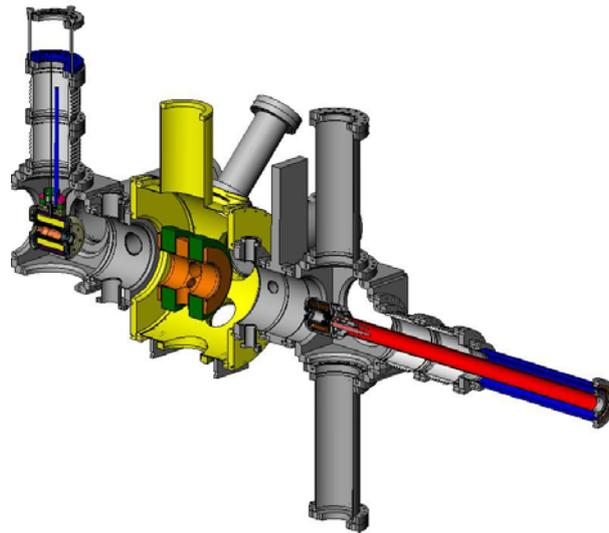
**FIGURE 8.** Heidelberg design study for the new TESLA/TRIUMF EBITs.
