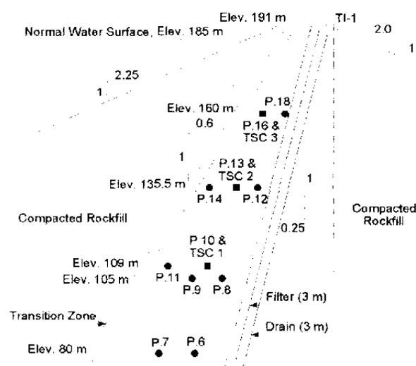
Fig. 1 Embankment geometry and instrumentation
