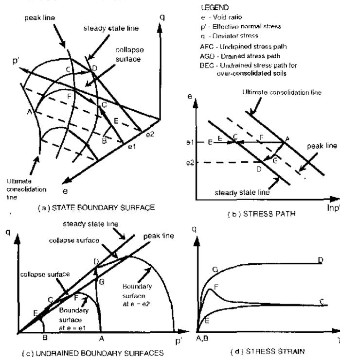
Fig. 1 State Boundary Surface For Loose Sands
