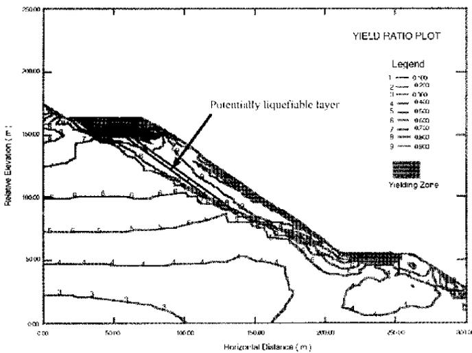
Fig. 4 Initial Yielding Ratio In Greenhills Cougar 7 Dump
