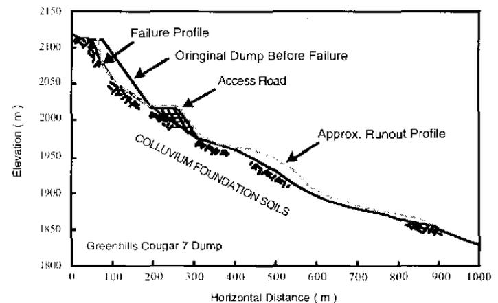
Fig. 2 Flow Failure of Greenhills Cougar 7 Dump
