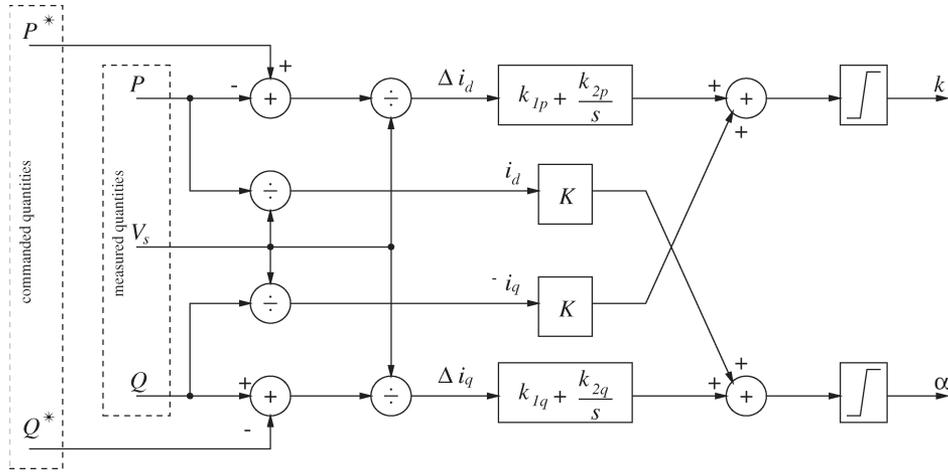
Fig. 7. Decoupled PQ control.
