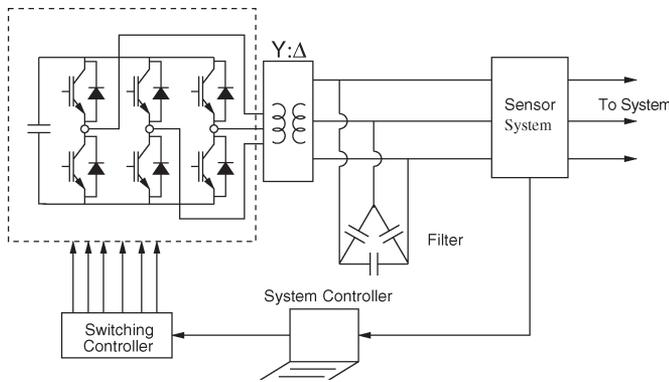
Fig. 1. Schematic of the traditional six-pulse STATCOM.
