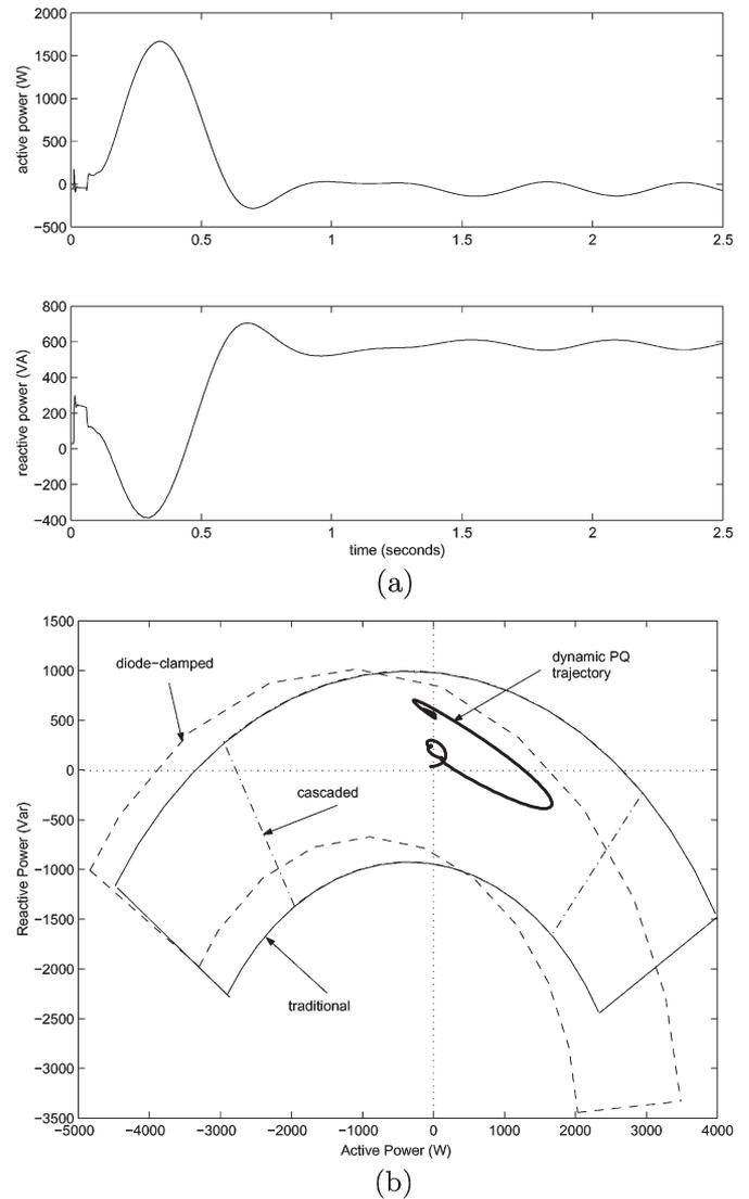
Fig. 10. (a) Time-domain simulation. (b) Operating range STATCOM active and reactive power injection.
