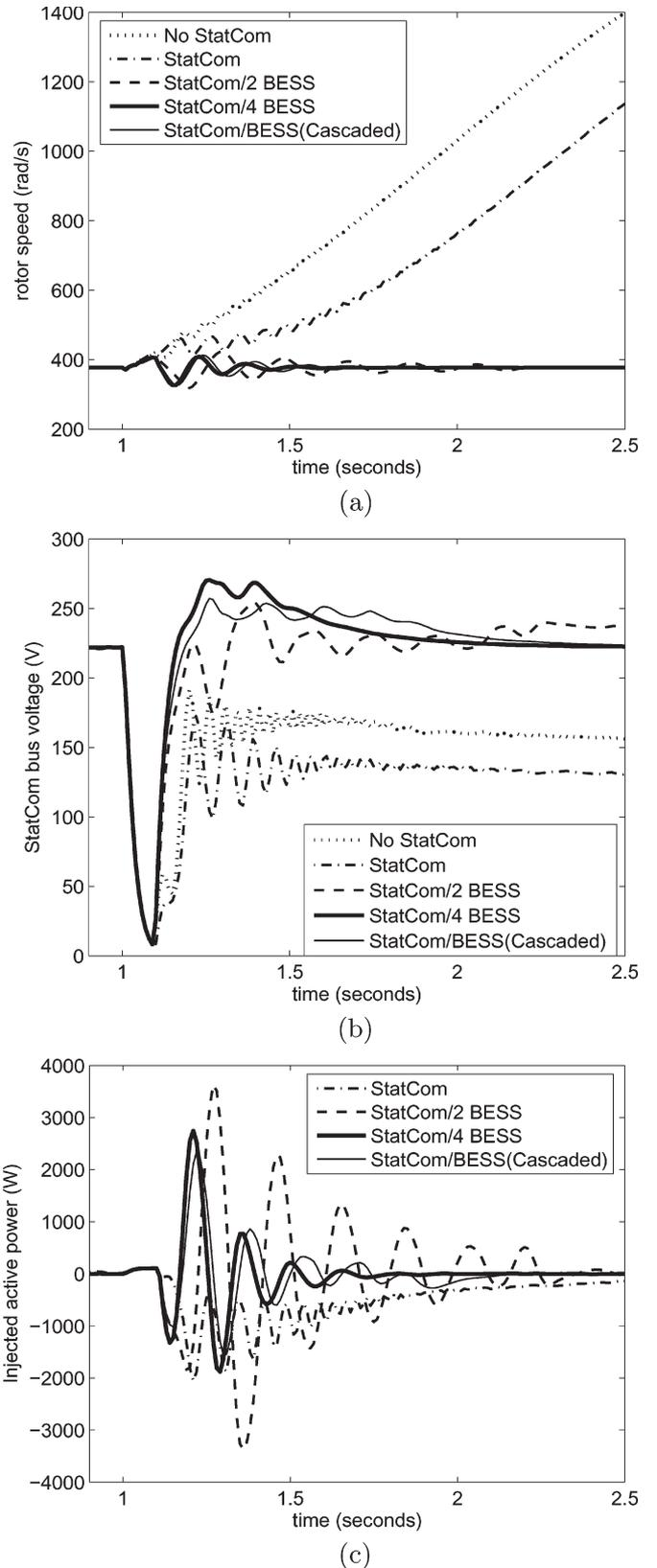
Fig. 11. Response to a 50-ms fault. (a) Rotor speed. (b) STATCOM bus voltage. (c) Injected active power.
