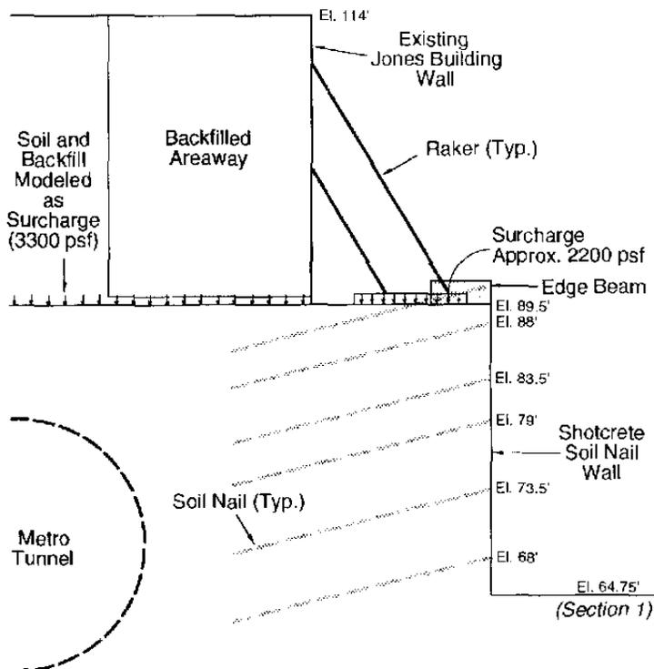
Fig. 4 Soil Nail Wall Section 1 at Jones Building
