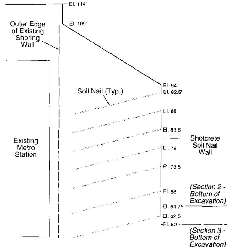
Fig. 5 Soil Nail Wall Sections 2 and 3 for Shallow and Deep Excavations at Station
