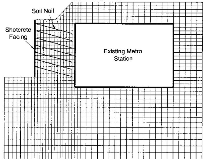
Fig. 2 *FLAC Model for Soil Nail Excavation*
