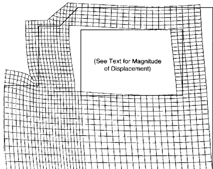
Fig. 3 *Deflected Mesh for Soil Nail Excavation*
