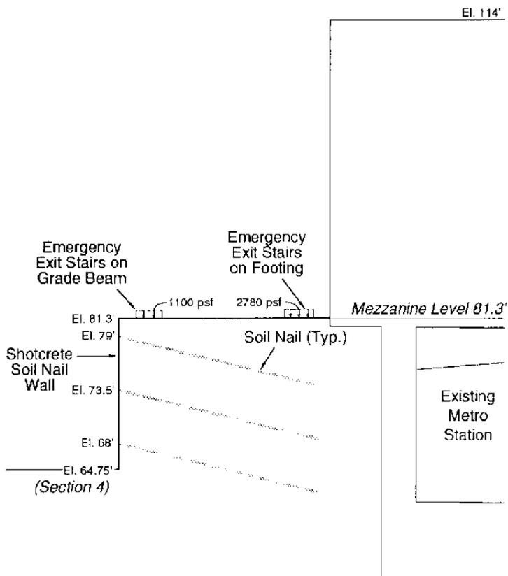
Fig. 6 Soil Nail Wall Section 4 at Station Entrance
